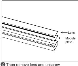
Then remove lens and unscrew module plate.
